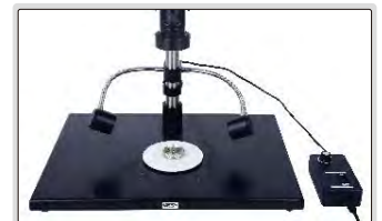
illumination direction and brightness are adjustable
