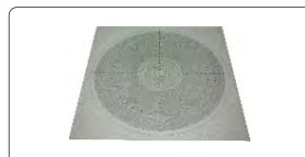
Ø300mm overlay chart (protractor with 1° graduation, radius with 1mm increment)
