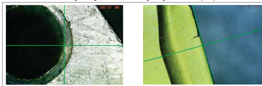
after finding the edge, the crosshair changes to green color and prompts
