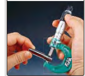
friction thimble for one hand operation
