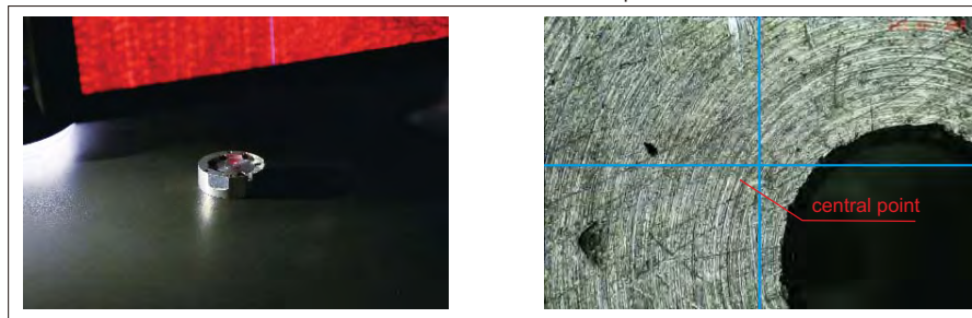
laser indicator locates the central point
