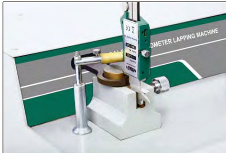
lapping measuring surfaces of caliper lower jaws
