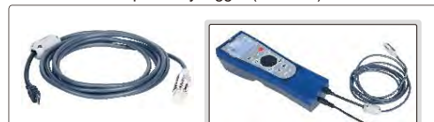
make LED flash frequency same as the rotation or vibration (power supply from AC/DC adapter when external trigger is used)
