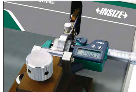
lapping measuring surfaces of outside micrometer
