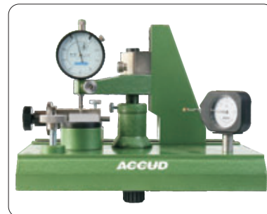
check the effect of lateral force on accuracy of dial indicators
