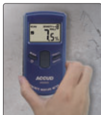
Measure concrete moisture
