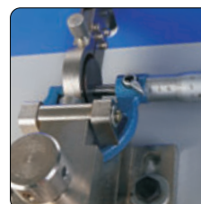
Lapping measuring surfaces of outside micrometer
