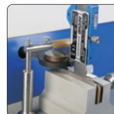
lapping measuring surfaces of caliper lower jaws
