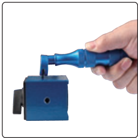
step 1: make grid cutting on surface
